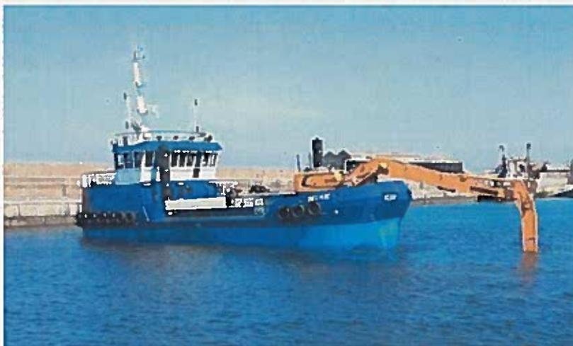
The MV Selkie is an efficient, highly manoeuvrable and cost-effective solution to a wide variety of dredging and associated marine projects.
